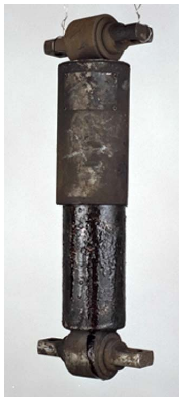
Wet Film Below Dust Cover With Defined Oil Droplets
