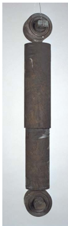
Moist Film Covering Entire Damper
