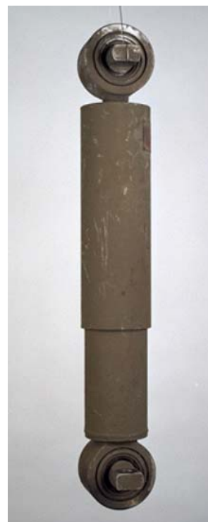
Damper with Road Dirt Accumulation
